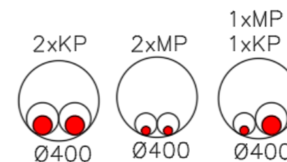
Installation of two cable in a Ø400 external protective pipe
